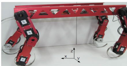
Figure 5. Dynarobin - a compliant quadruped robot design 1 .
