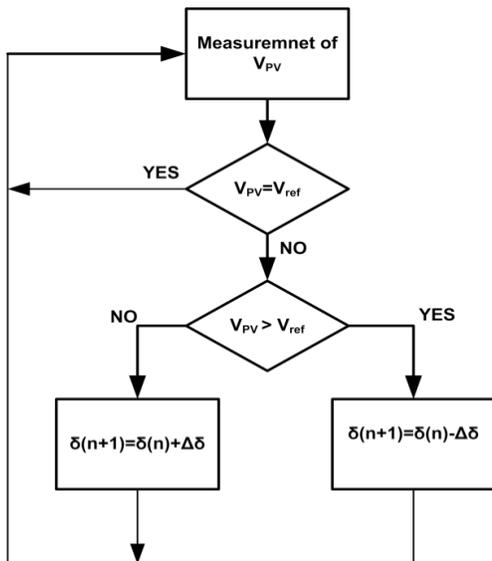
Figure 1. Flow chart of the CV method.
