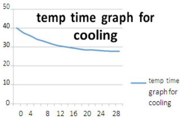
TEMPERATURE-TIME GRAPH FOR COOLING OF 50°C WATER
