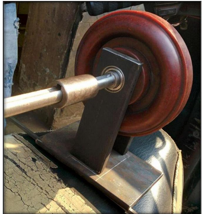
Figure 5. Rear Wheel with shaft, bush and keyway.
