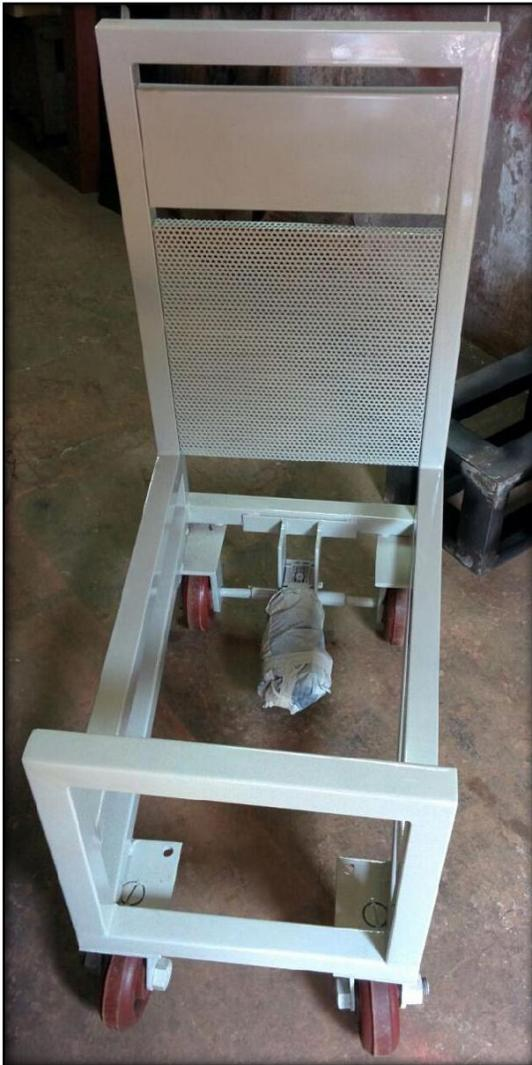
**Figure 7.** Trolley Sub Assembly.
