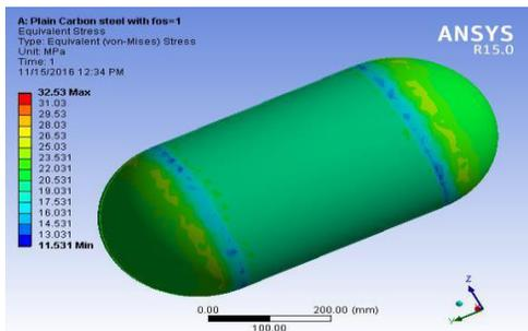
Figure 4. Equivalent stress on steel gas cylinder.
