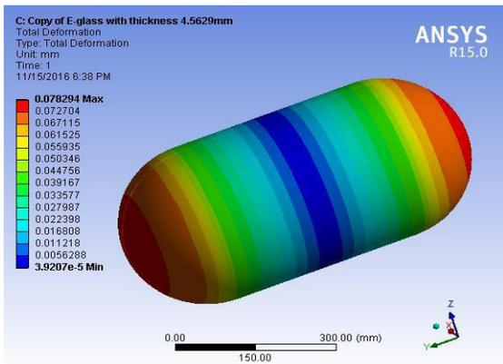
Figure 9. Total deformation of E-glass gas cylinder.
