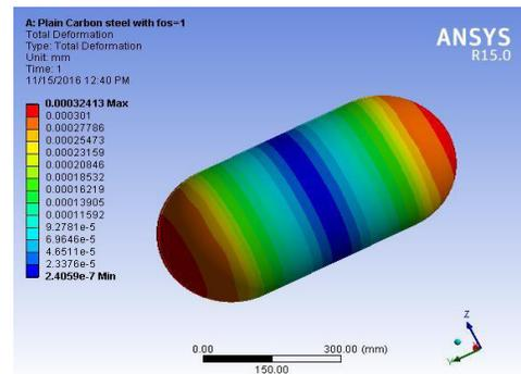
Figure 8. Total deformation of Steel gas cylinder.
