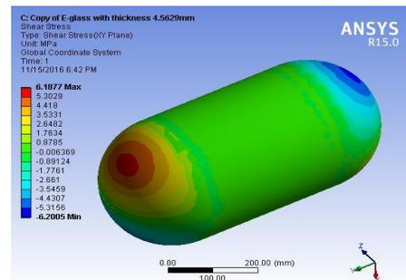
Figure 7. Shear stress distribution of E-glass gas cylinder.
