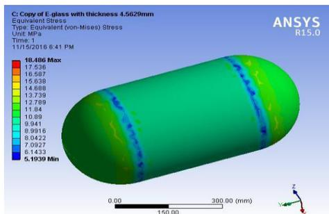
Figure 5. Equivalent stress on E-glass gas cylinder.
