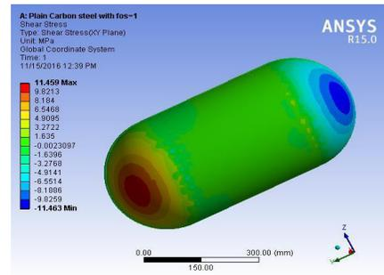
Figure 6. Shear stress distribution of steel gas cylinder.
