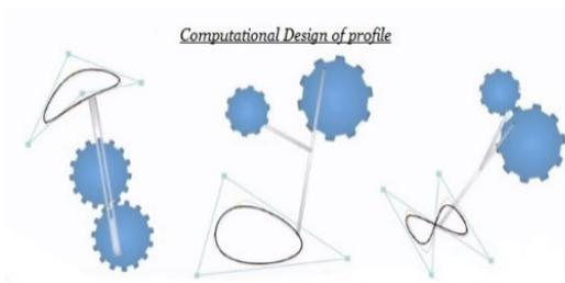
**Figure 1.** Computer generated profile using 2-gear method.
