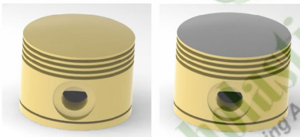
Figure 3. 3D model of piston without and with TBC Coating.
