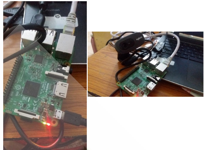
Figure 5. The setup made to run the experiments for facial detection and recognition. The first picture shows the Raspberry Pi board while the second picture shows the whole setup along with the webcam.
